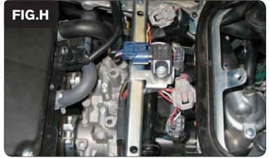
12 Plug the PCV connectors in-line with the fuel injectors and stock wiring harness (Fig. H).
