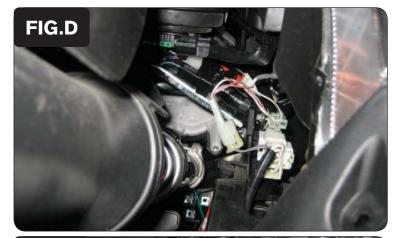
7 Plug the PCV in-line of the stock crank pickup coil connectors (Fig. D).
