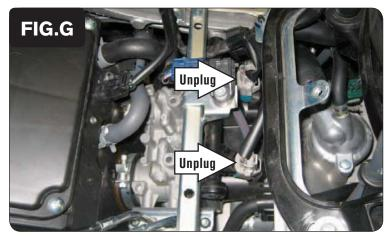
11 Locate the fuel injectors (Fig. G).
