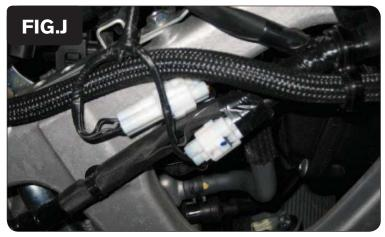
14 Plug the PCV wiring harness in-line of the stock TPS connectors (Fig. J).
