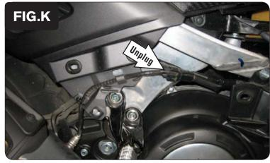
15 Locate the stock O2 sensor connection and unplug it (Fig. K).
