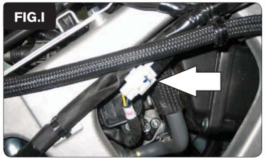
Locate the 3 pin white sub-connector of the Throttle Position Sensor on the external right side of the frame (Fig. I).
