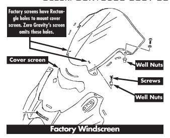
Factory cover screen is not transferred to Zero Gravity screen. Factory transferred parts are the Well Nuts and screws. If factory Well Nuts are deformed (as shown right) you may want to change them out with our ZG Well Nuts kit part #32-111.
